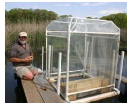
A new facility for studying the interactions of elevated CO 2 , sea level rise and nitrogen pollution.
