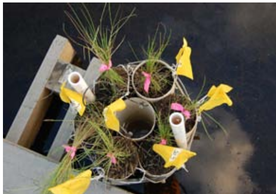
Top view of a "marsh organ", used to manipulate sea level.
